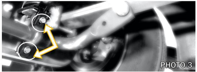
Remove two bolts from drivers (PHOTO 3) and install the B1058 axle bracket with the round end upwards and angle towards the rear.
